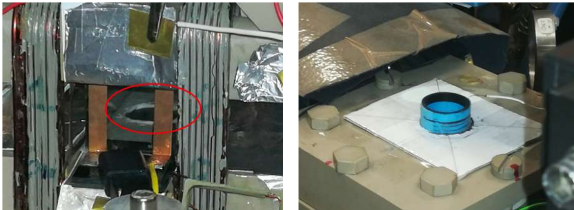
Figure 2.8: On the left side, a close-up photo of the bottom mesh seen between the frontal ionization plates and through the cell (The Aluminium plates mentioned in section (2.6.3) are already placed). On the right side, a photo of the upper part of the tube that sustains the top mesh. Note the ticks that allowed us to adjust the distance between the upper mesh and the cell with a precision of about 1 mm.
