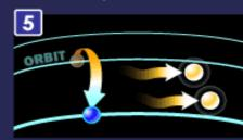
...produces two photons of the same wavelength and phase.
